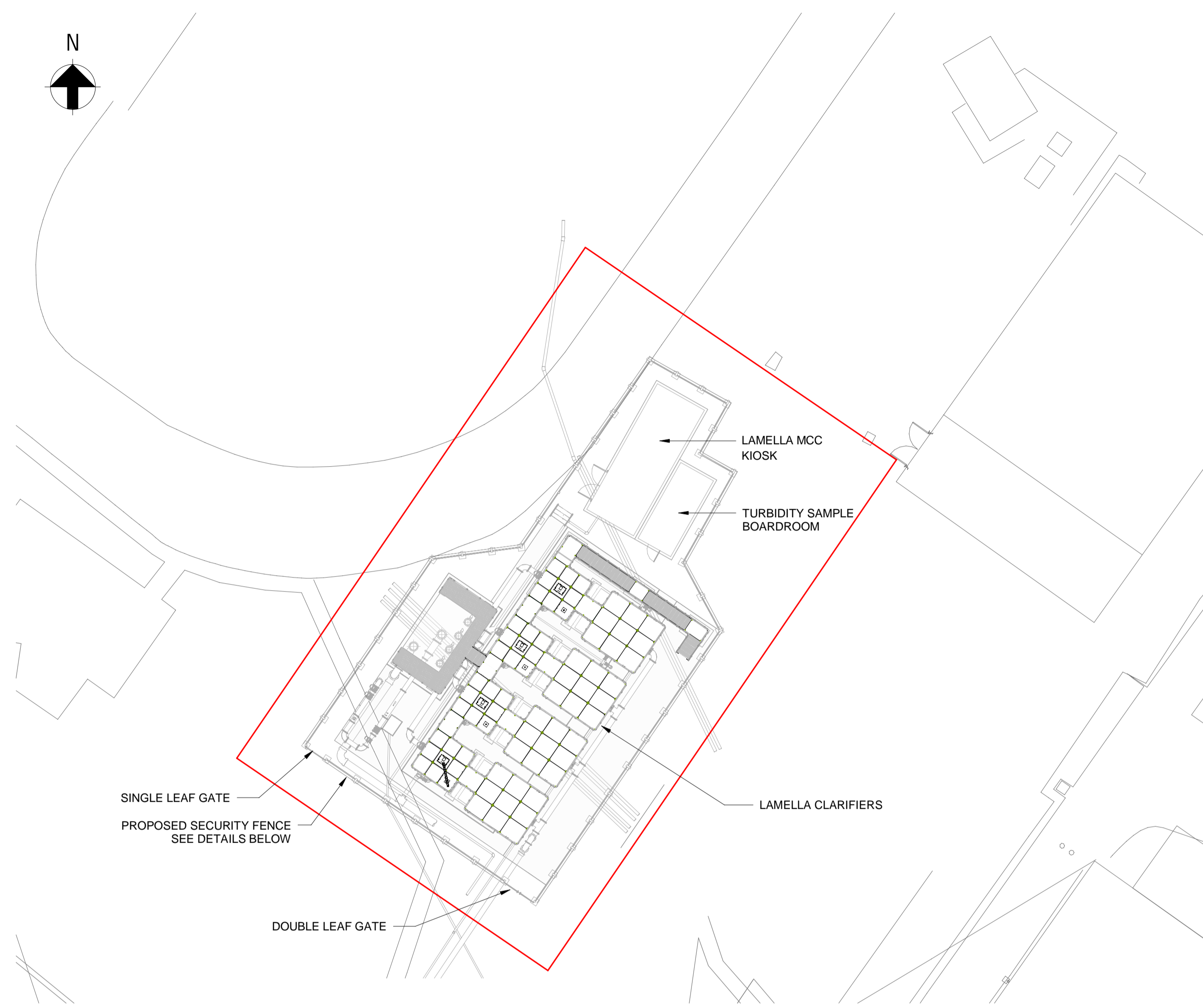
LAMELLA FENCING AND MCC KIOSK PLAN 1 : 200
