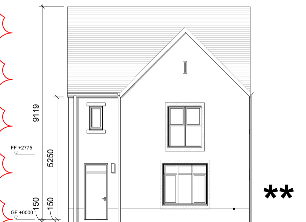
FRONT ELEVATION - PLOT NO. 73, 80, 81 (DARK BRICK) PLOT NO. 74, 75, 82 (RENDER WITH LIGHT BRICK BASE AND DETAIL)
