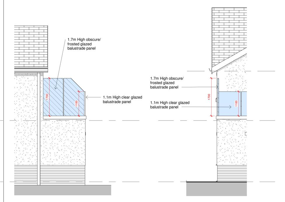
Typical Proposed Balustrade Side Elevation
