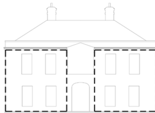
Symmetrical layout of elevation incorporating square bays either side of a central door or feature
