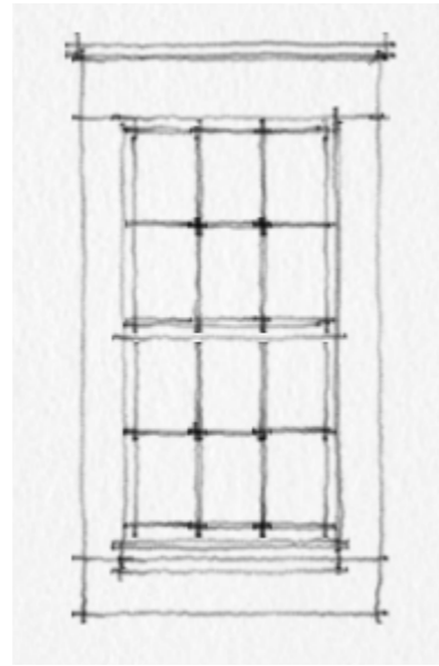
Stone heads and jambs with sliding sash window, Whins House, Sabden
