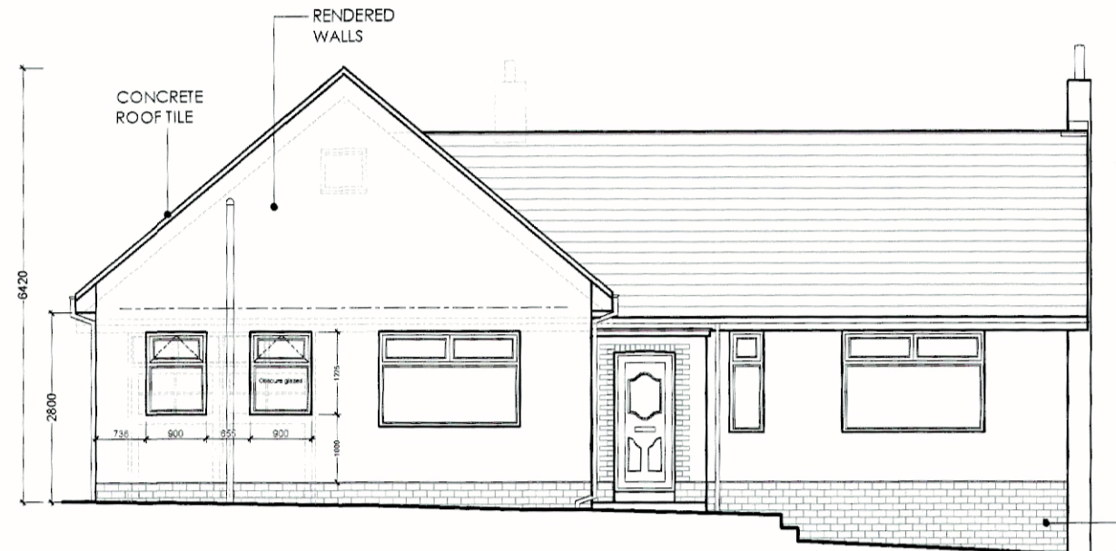
PROPOSED NORTH EAST FACING ELEVATION SCALE 1:100
