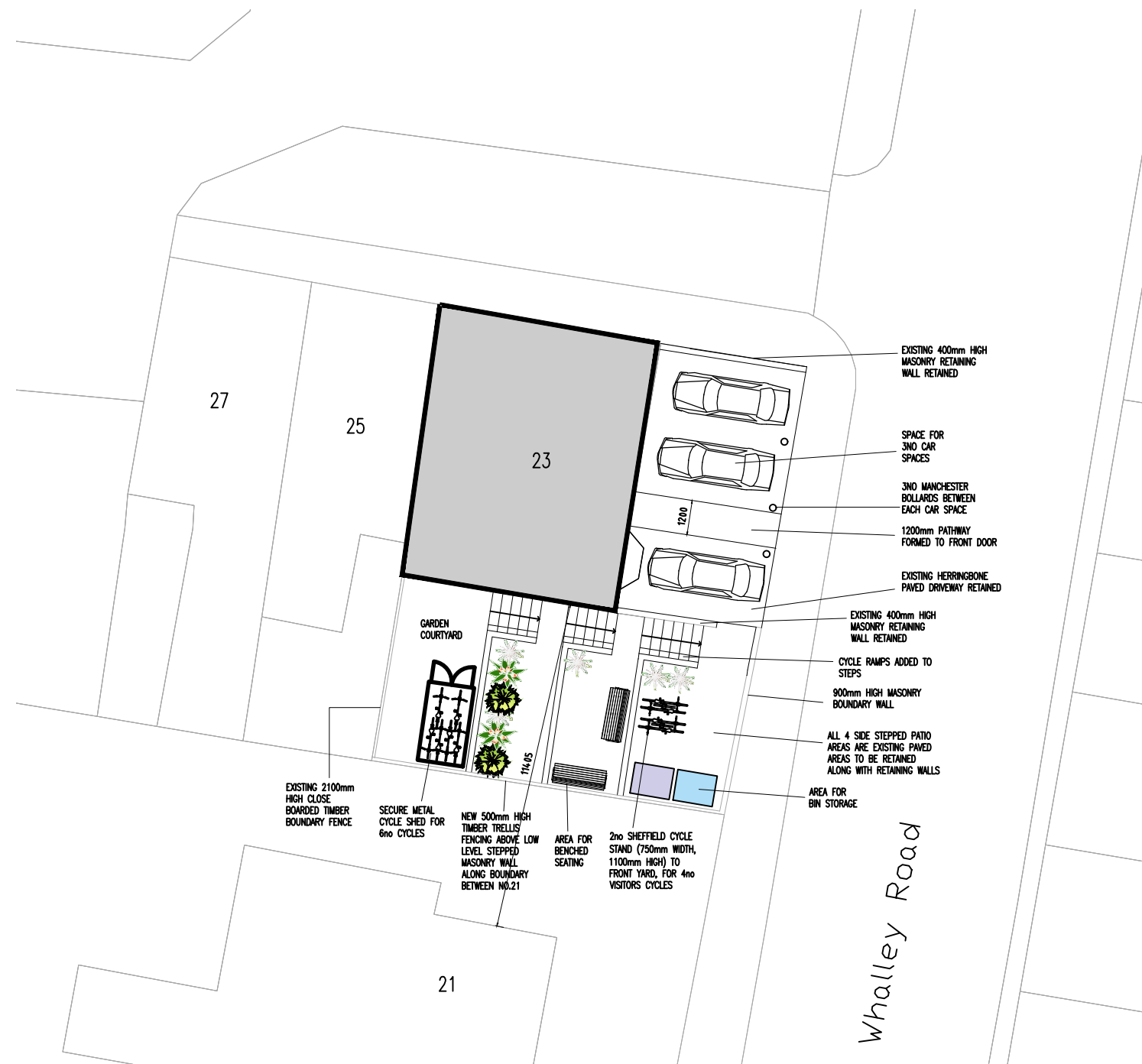
PROPOSED BLOCK SITE PLAN 1:200@A3
