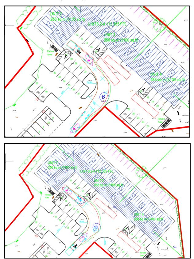
If unit 3 and 4 occupied, unit 2 enters in forward gear and loads etc from rear, exits as shown below.
