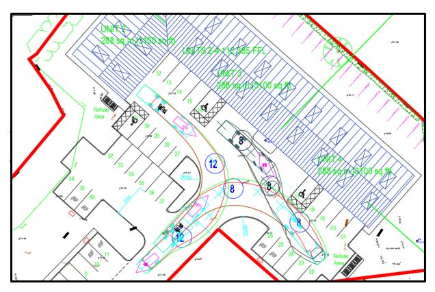
Unit two occupied, unit three enters and reverses into middle loading area, unit 2 can exit.
