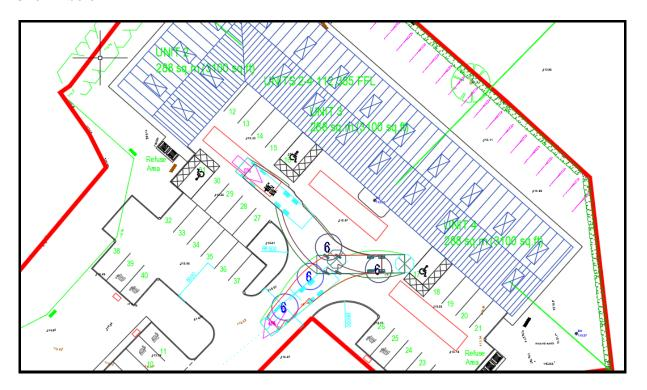
Furthermore, the LHA require another tracking drawing showing that two-way movements between an HGV and a vehicle can be undertaken simultaneously along the internal carriageway within the site. This is because the LHA are concerned that should an HGV be using the internal carriageway it may be too narrow for two-movements to occur. Therefore, the LHA require further evidence to ensure that the width of the internal carriageway is suitable for the site.
