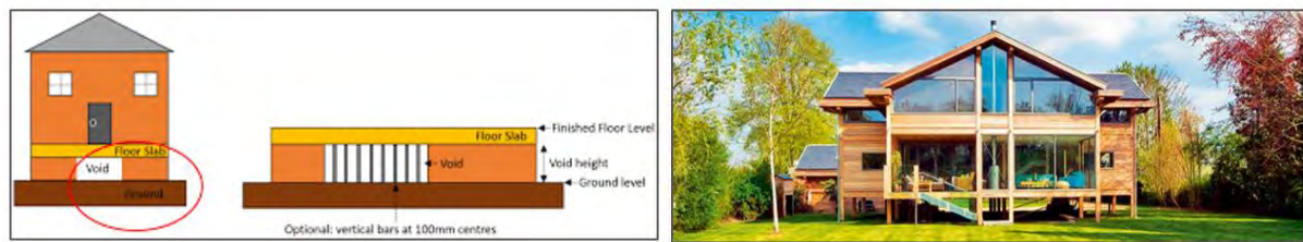
Figure 7. Schematic of theory behind the use of voids for floodplain storage
