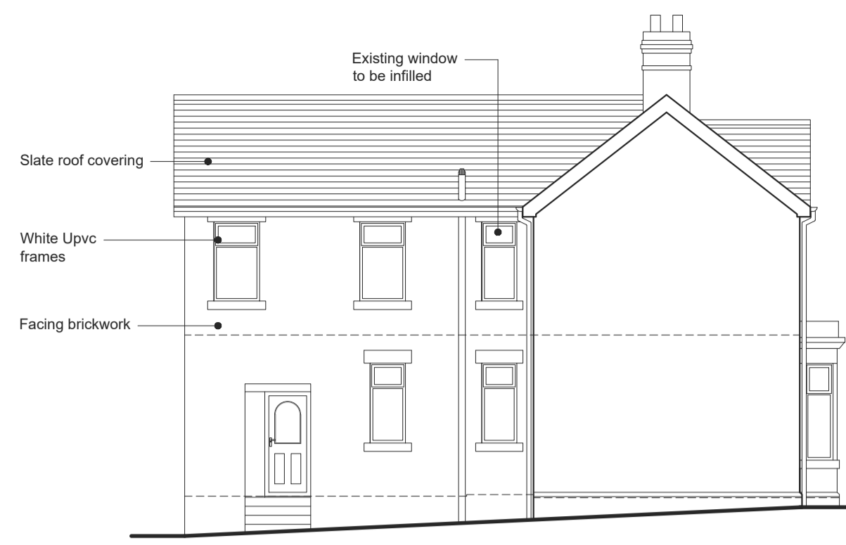
EXISTING SOUTH WEST ELEVATION Scale 1:100
