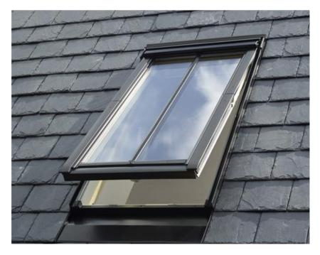
The proposed rooflight to be a Velux conservation rooflight 550 x 980mm, Ref: CK04. Rooflight to be top hung, flush fitting. External finish to be black aluminium with central glazing bar. To be complete with recessed installation flashing kit and include vapour barrier, insulation collar and under felt collar.
