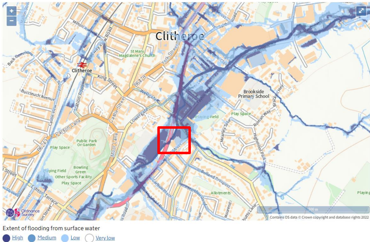
Figure 2.2 - Risk of Flooding from Surface Water Mapping
