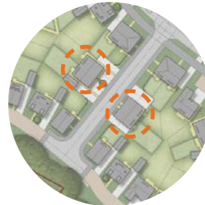
Excerpt from the previously submitted site layout showing the extent of the vehicular accessways crossing the 3m cycle way
