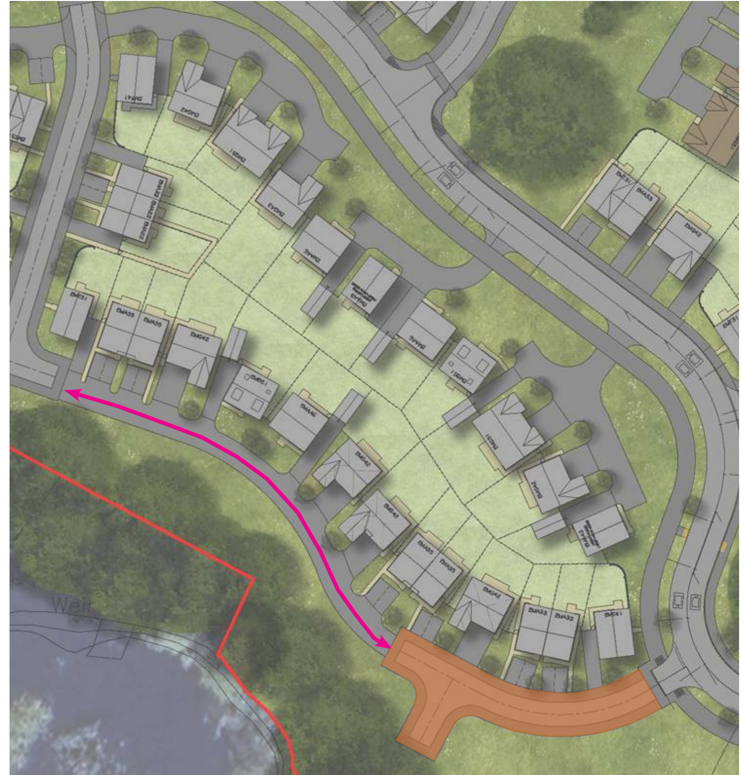
Excerpt from the current design iteration showing the reorientation of the parcel and linked private drive
