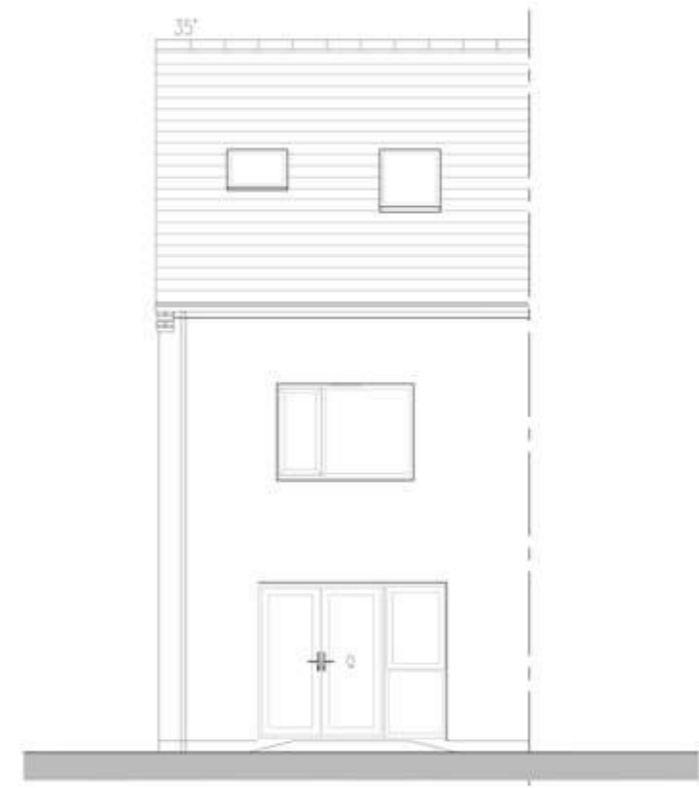
REAR ELEVATION END/SEMI DETACHED
