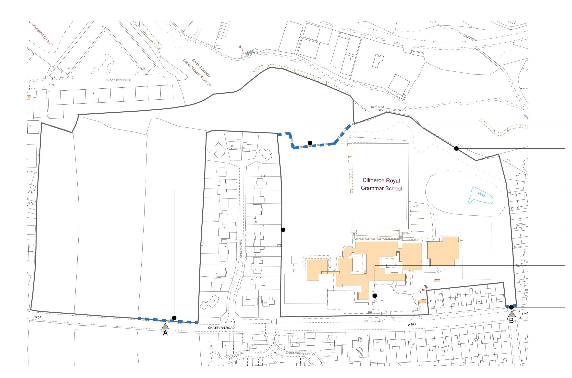
Supply and fit new 2.4m high weldmesh fencing along the boundary line. Supply and fit 1No. Double leaf vehicular access gate.
