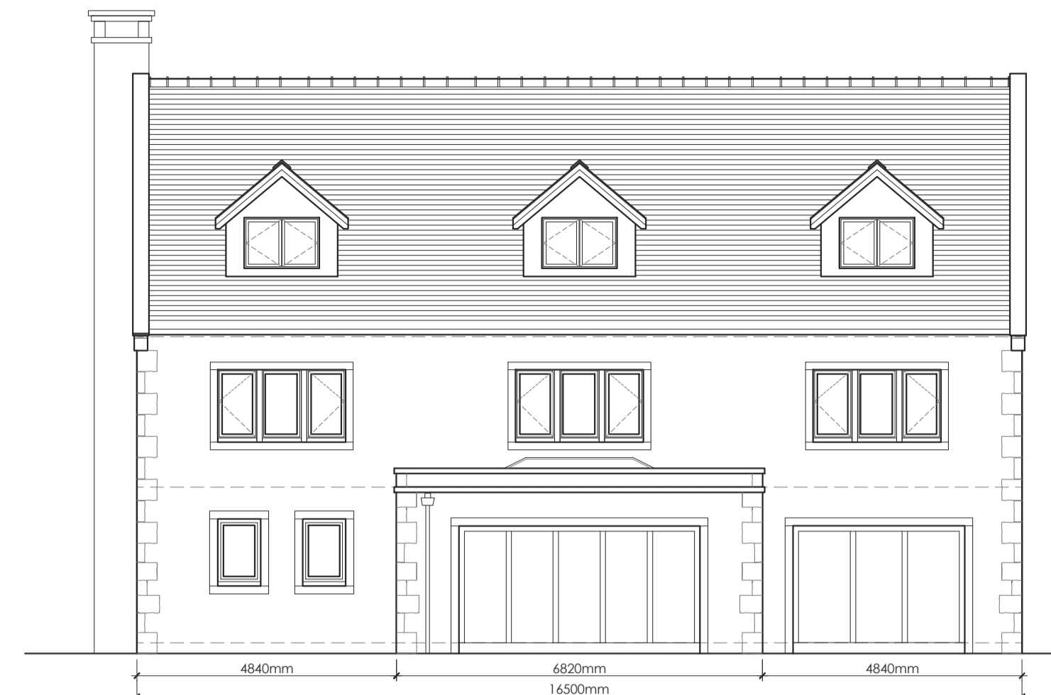
PROPOSED NORTH ELEVATION Scale 1:100
