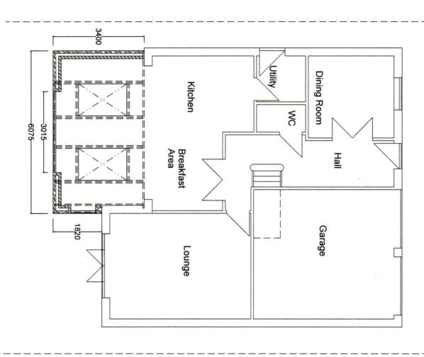
Proposed Atrium Extension to be Glass Flat Lantern Roof X 2 on Flat Warm Roof on White PVC Glazed Frames on Matching Face Brick Walling
