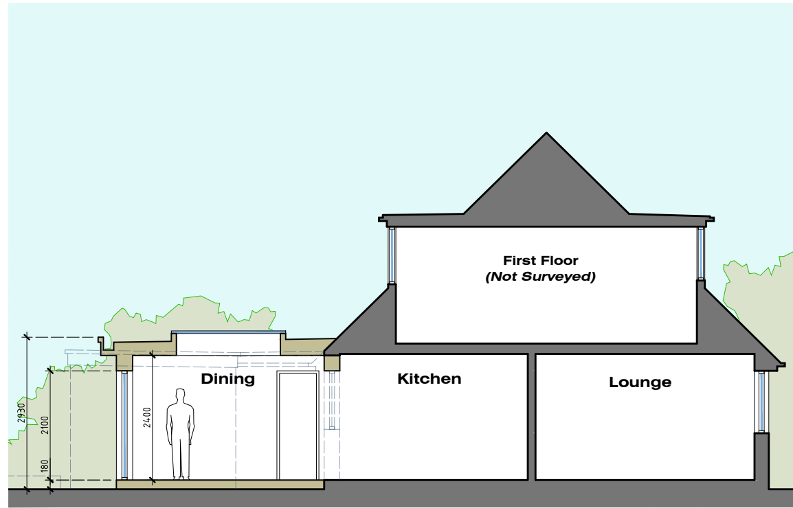
Side (South-East) Sectional Elevation
