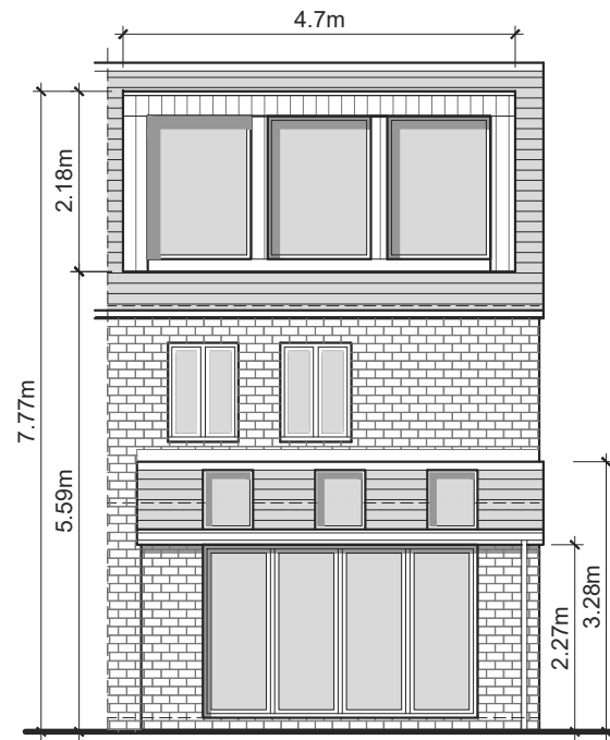
PROPOSED SOUTH ELEVATION Scale 1:100
