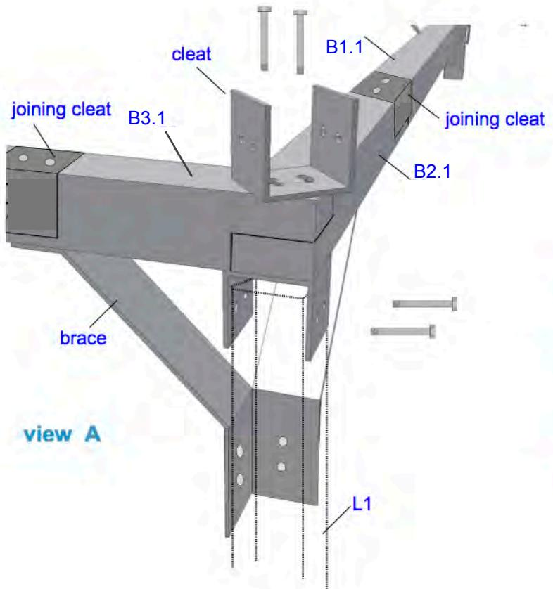
Stainless steel nuts can very occasionally weld themselves to the bolt thread and prevent tightening or removal. To reduce this we include copper anti seize compound. **Before attaching the nut it is essential to smear, about the size of a pea, to the end of each bolt thread and to the full length of the 4 x M10 bolts used for the canopy adjusters**
