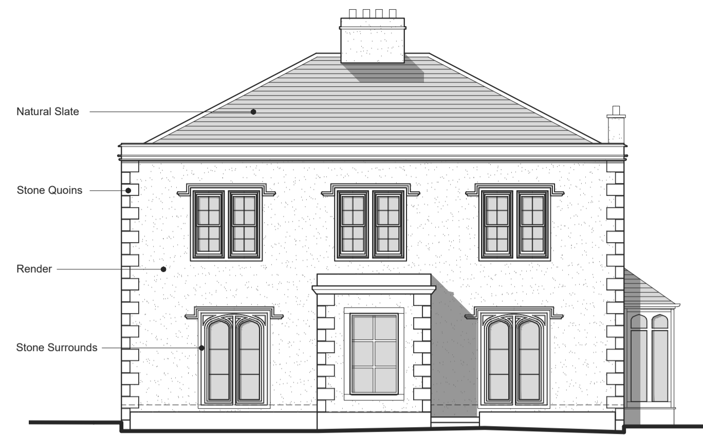
EXISTING SOUTH WEST ELEVATION Scale 1:100
