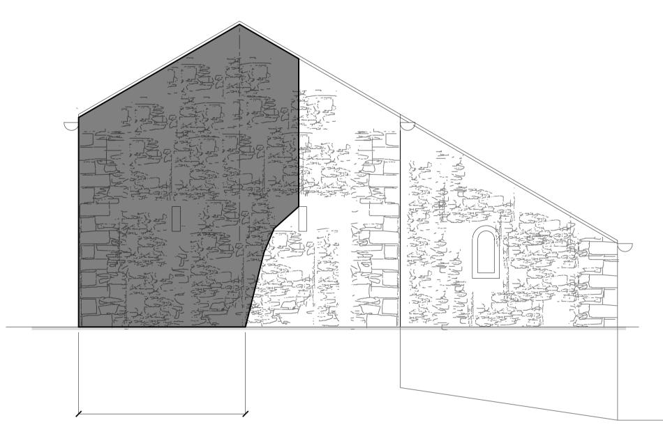
SECTION OF EXISTING WALL TO BE DEMOLISHED FULL HEIGHT AND RE-BUILT OFF NEW CONCRETE STRIP FOUNDATION FOUNDATION TO BE FORMED IN NATURAL GROUND CAPABLE OF SUPPORTING 100 kN/m<sup>2</sup>
