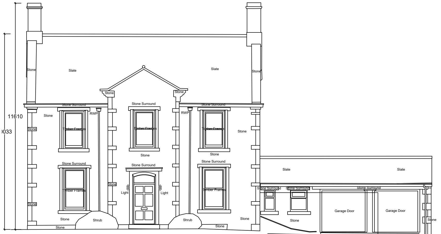
EXISTING FRONT ELEVATION SCALE 1:100
