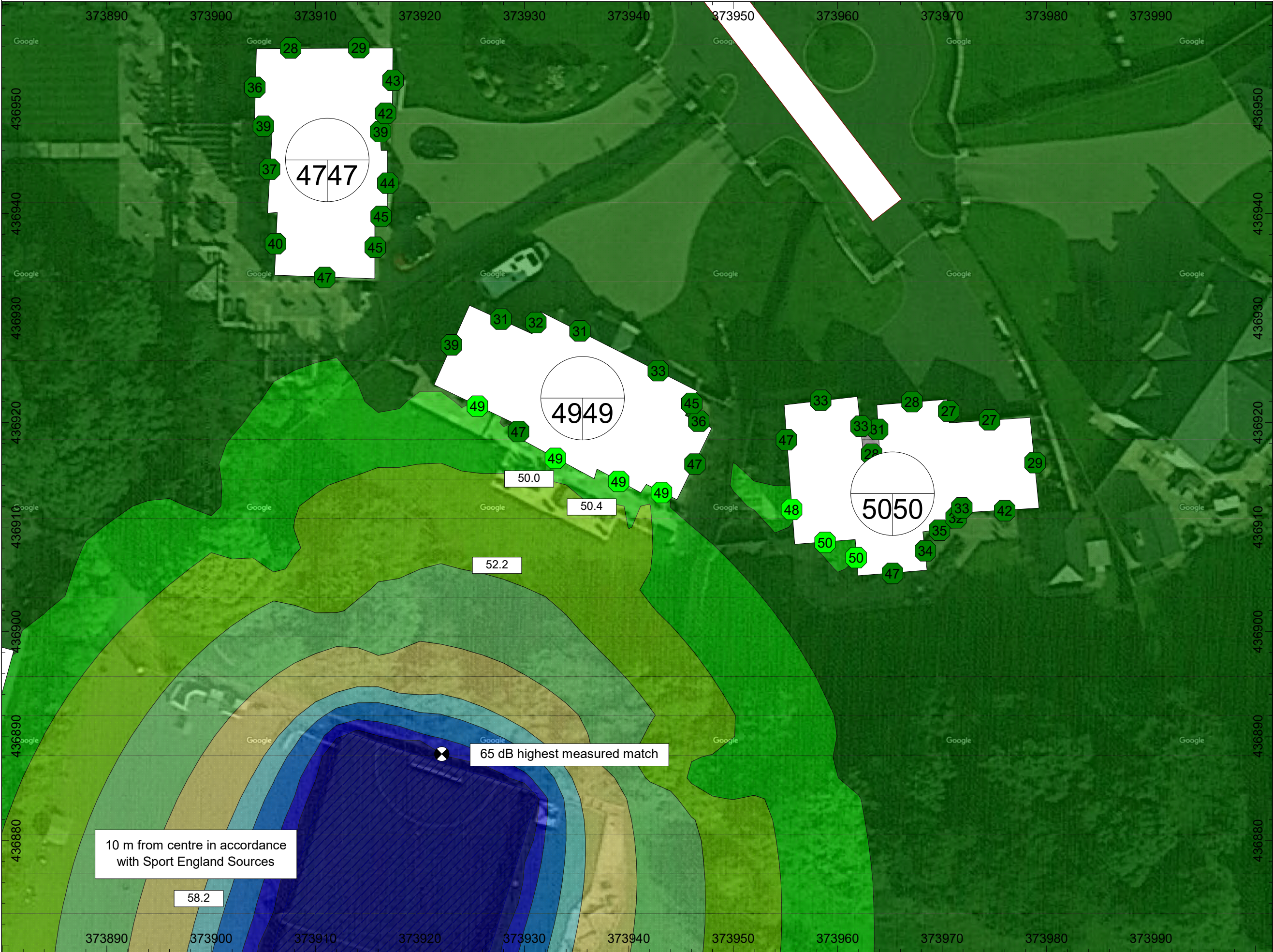
Figure 1 - Daytime Grid Noise Map - Calculation at 1.5m above ground level
