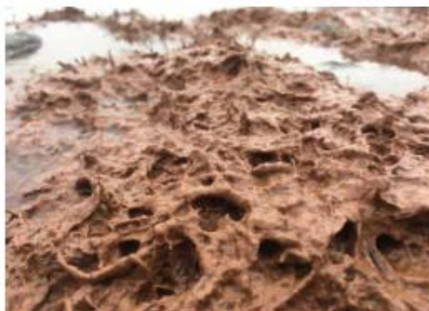
Close up FlocMat showing accretion of silt
