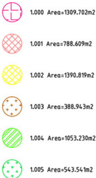
Fig1. Actual impermeable area drained by pipe.
