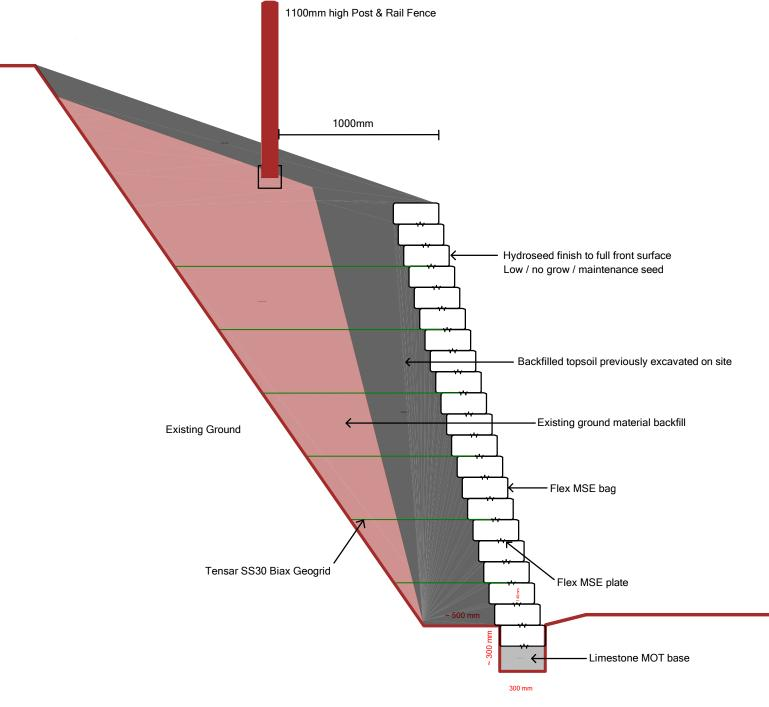
Existing ground - Stiff Clay, Clayey Gravel of Sandstone, Mudstone and Limestone with Boulders
