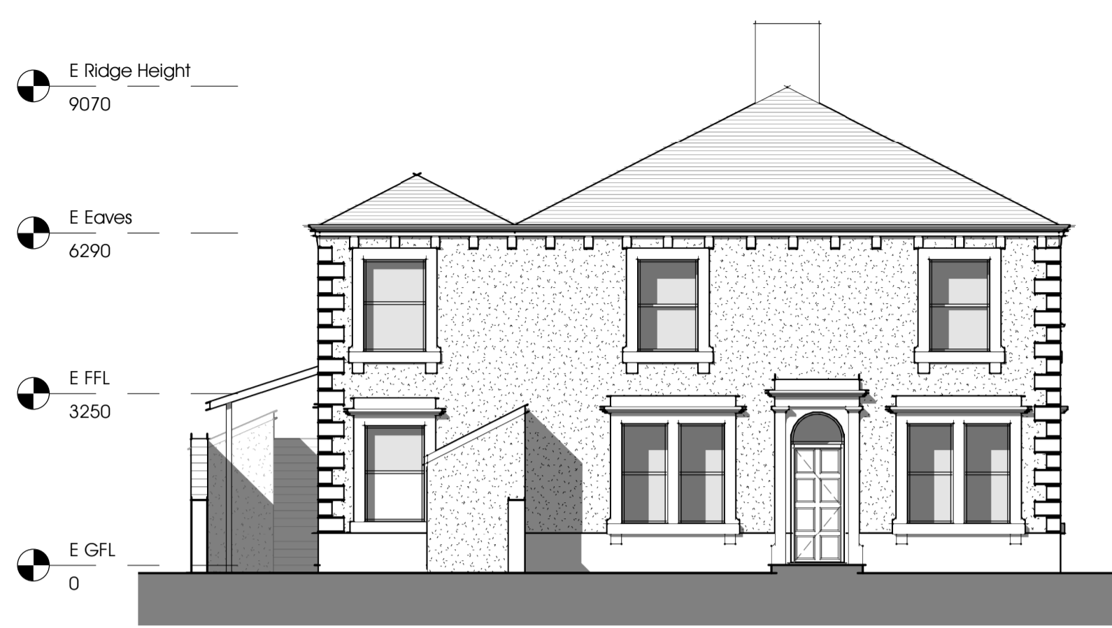
E1 Existing Front Elevation (South) 1 : 100
