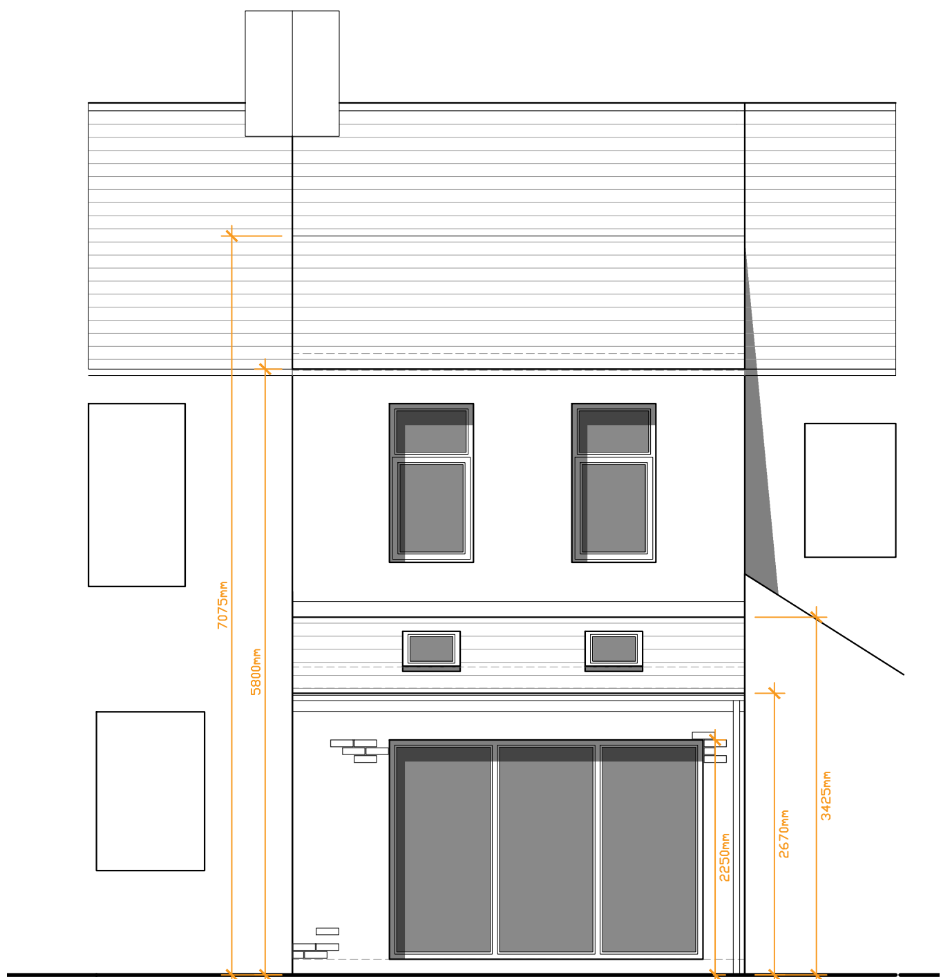
PROPOSED REAR (SOUTH WEST) ELEVATION Scale 1:50
