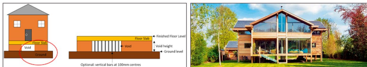
Figure 10. Schematic of theory behind the use of voids for floodplain storage
