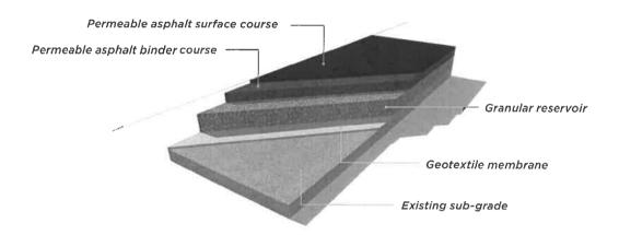
With all asphalt pavements the surface course is designed to provide a smooth finish, with no trip hazards an appropriate level of slip and skid resistance. These characteristics in a permeable solution are maintained whilst being free draining (removing risks of standing water and ice) and acting as a pollutant filter, removing contaminants prior to discharge.
