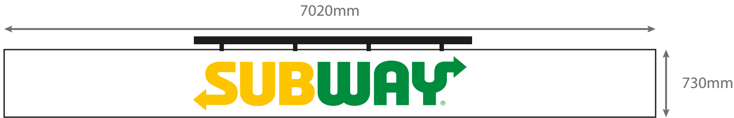
Folded P/C Aluminium sign tray with S/A Vinyl letters overhead trough light
