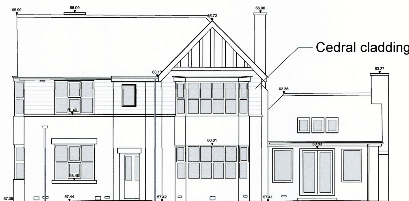
▼ 55.00m above OS Datum South Elevation 1:100 Scale
