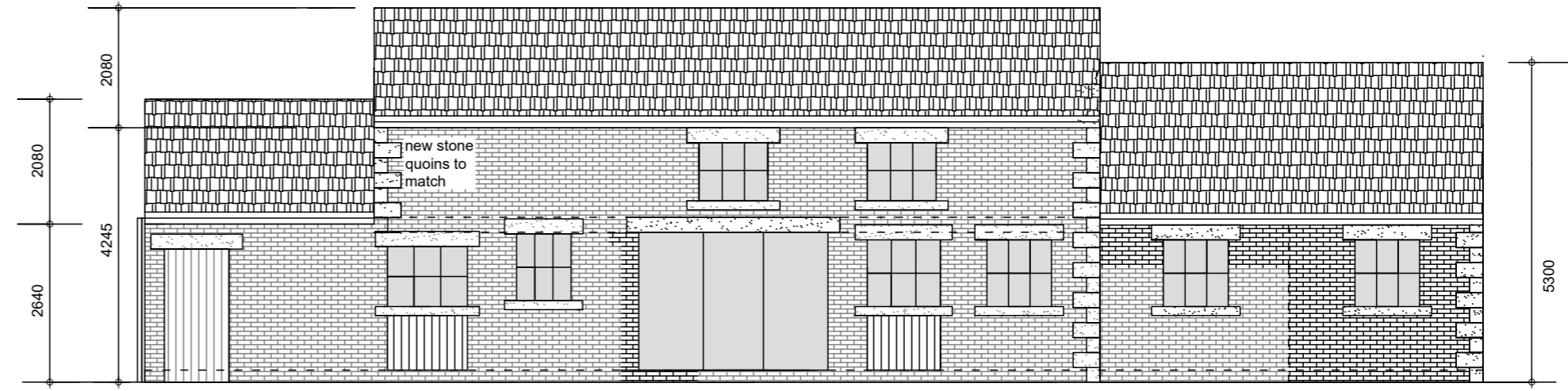
PROPOSED NORTH EAST ELEVATION (1 : 100)
