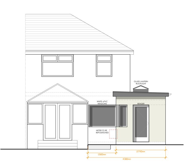
PROPOSED REAR (NORTH) ELEVATION -Scale 1:50
