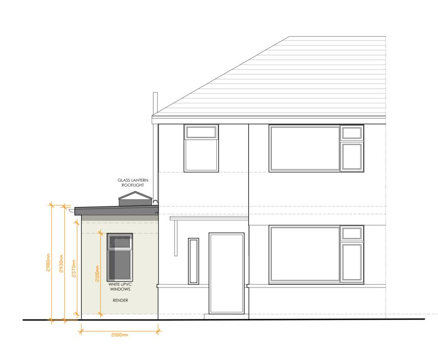
PROPOSED FRONT (SOUTH) ELEVATION - Scale 1:50
