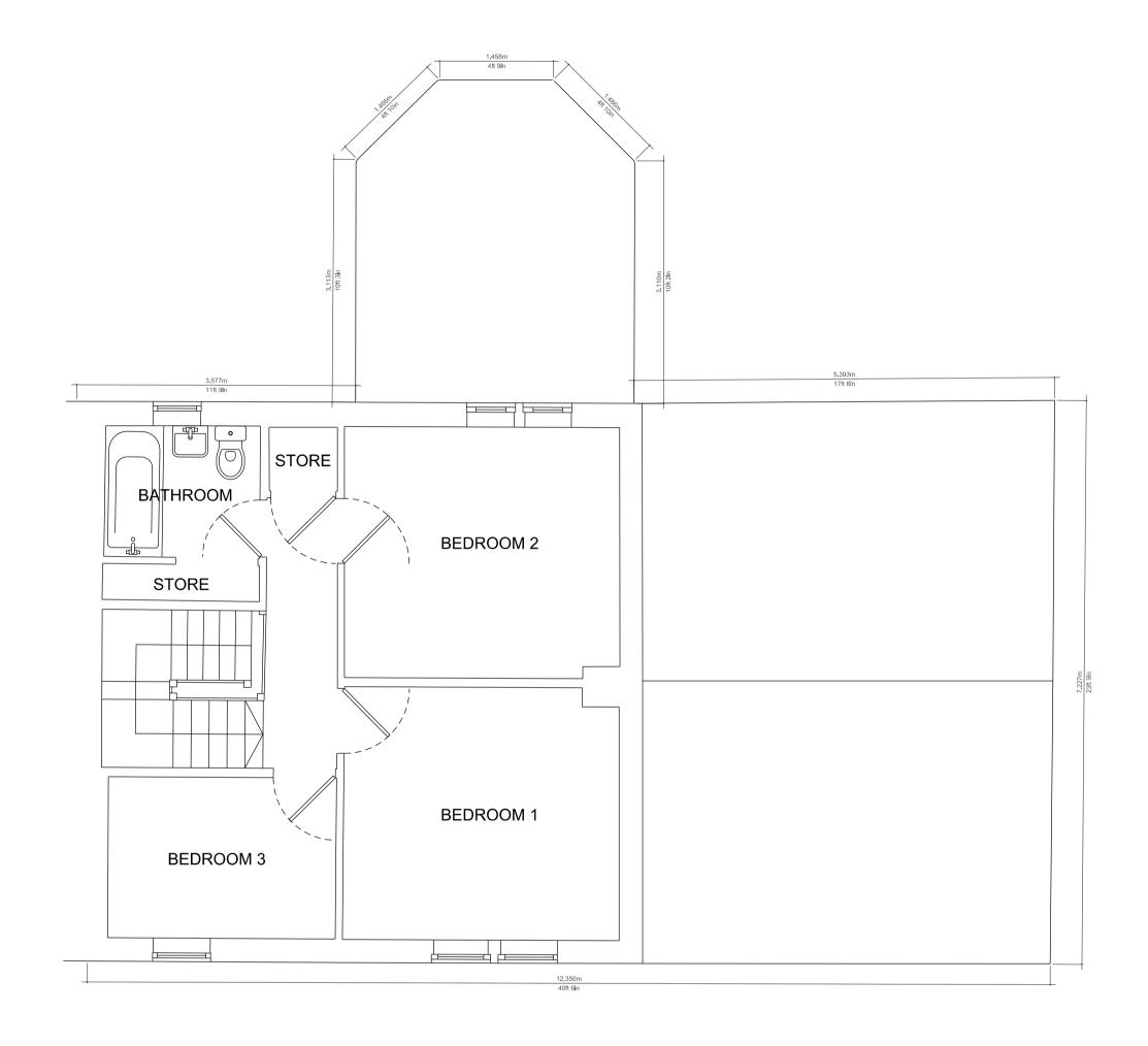
Existing First Floor Plan Scale 1:50
