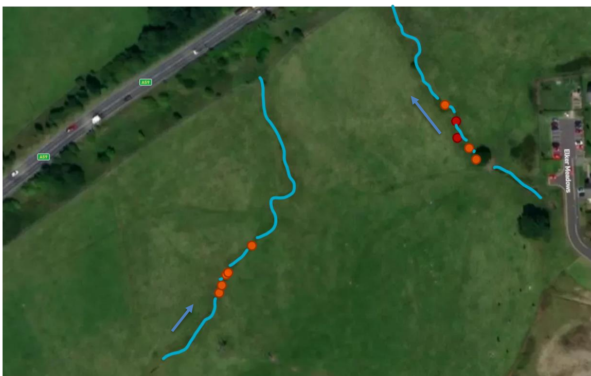
Figure 4.1: Aerial view of the Elker Lane West (ELW) and Elker Lane East (ELE) streams in Land off Elker Lane in blue (arrow indicates flow direction). The 10 cross section survey locations (MoRPh 1 to 5 ELW and 1 to 5 ELE) are marked by red and orange dots. Map from Cartographer Copyright Mapbox, OpenStreetMap and Maxar.
