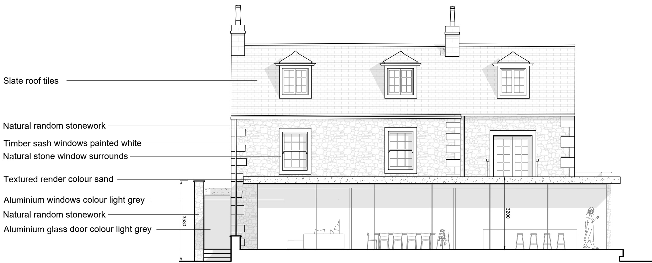
Proposed South Elevation Scale 1:100
