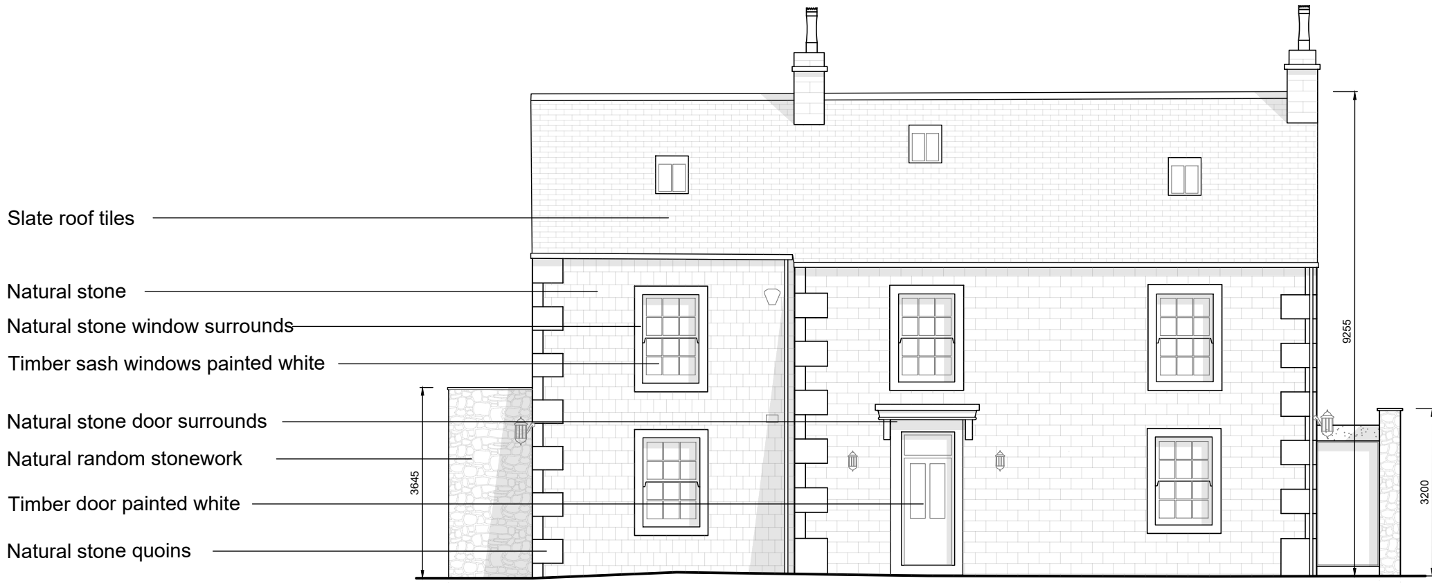
Proposed North Elevation Scale 1:100
