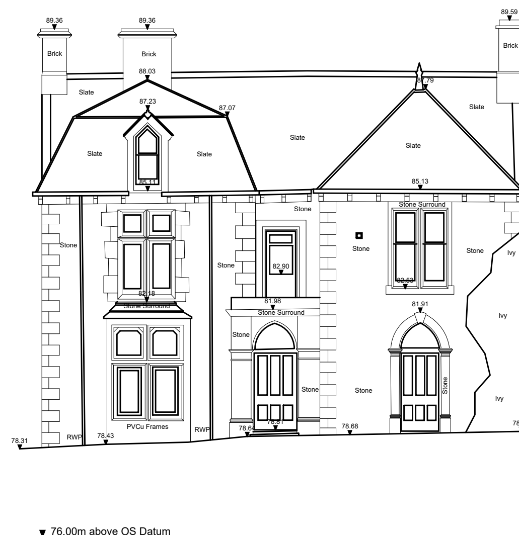
North West Elevation
