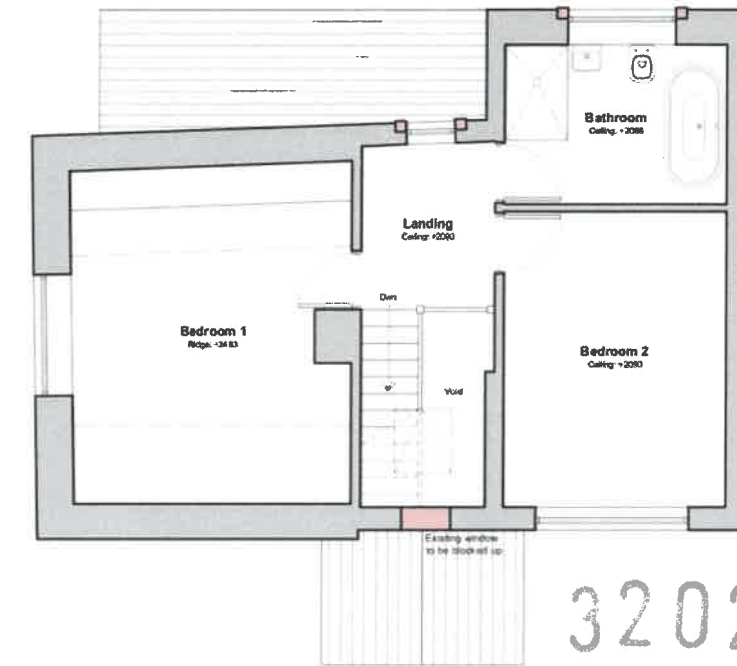
Proposed First Floor Plan Scale 1:100
