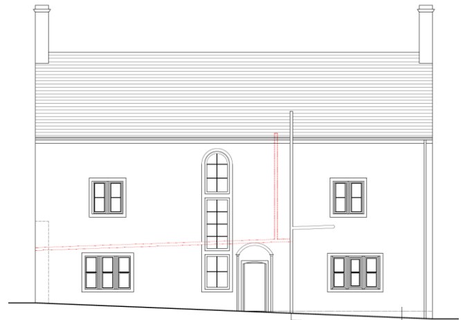
PLI 3: Proposed rear north elevation showing the location of the proposed soil stack and the removal of the existing soil stack and waste branch.
