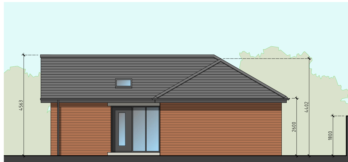
Side/ Sectional (East) Elevation
