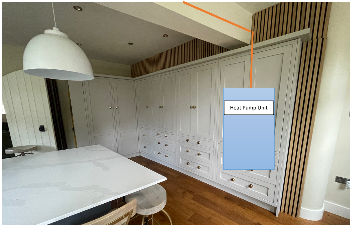
Modern internal panelling and ceilings and an illustration of where the heat pump and connecting pipework will be installed behind these modern panels.
