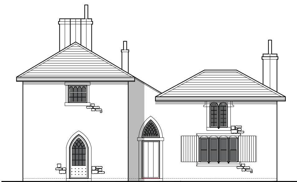
EXISTING EAST ELEVATION SCALE 1:100 0 2 4 6m
