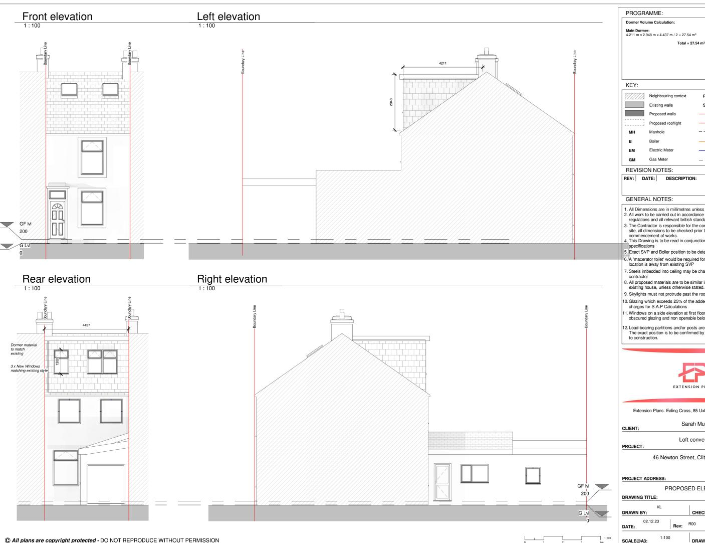
PROGRAMME: Dormer Volume Calculation: **Main Dormer:** 4.211 m x 2.948 m x 4.437 m / 2 = 27.54 m<sup>3</sup> Total = 27.54 m<sup>3</sup>
