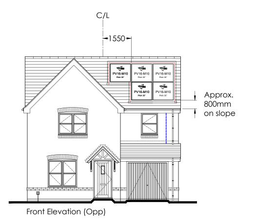
Fusion Roof Integrated PV Array 5 No. PV16-M10 Panels Mounted in Portrait Orientation
