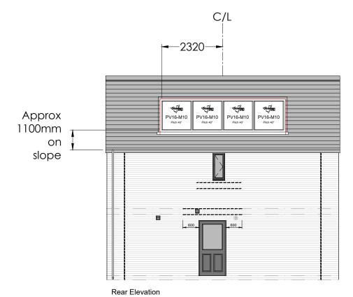
Fusion Roof Integrated PV Array 4 No. PV16-M10 Panels Mounted in Portrait Orientation
