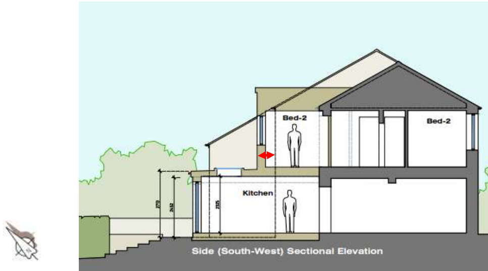
PROPOSED SECTIONAL ELEVATION SHOWING MODEST 0.7 METRE PROJECTION OF FIRST FLOOR EXTENSION OF No 67 BEYOND REAR WALL OF No 69.
