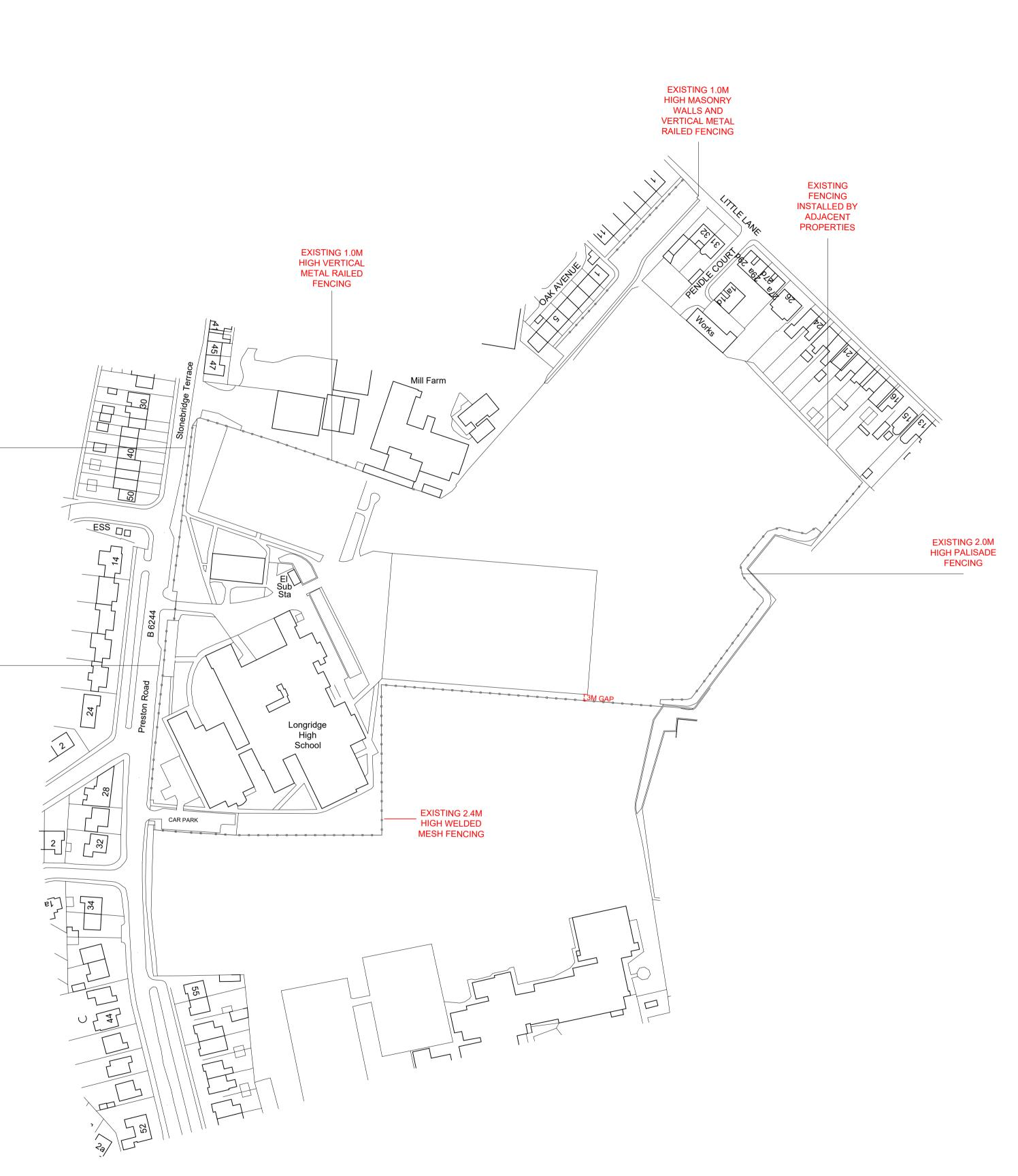
EXISTING 1.0M HIGH MASONRY WALLS AND VERTICAL METAL RAILED FENCING
